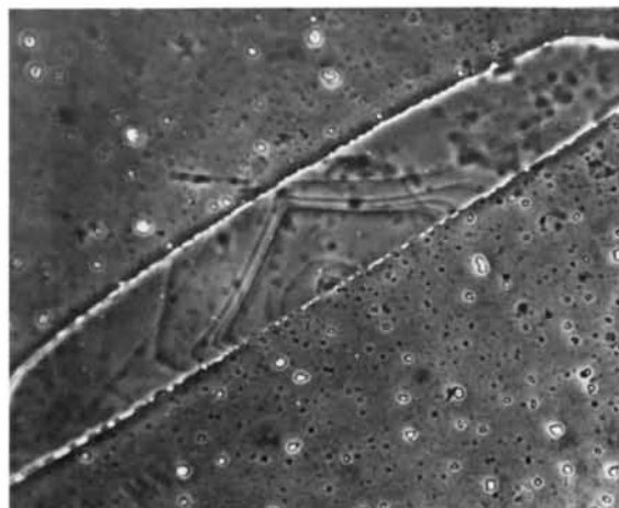
Fig. 2. Crystal of n\text{-C}_{34}\text{H}_{70} showing the same development as in Fig. 1(a). The micromorphology of the upper face exhibits in this instance a coalescence of growth steps having their mutual orientation rotated \pm 90^\circ with respect to that of Fig. 1(a).
